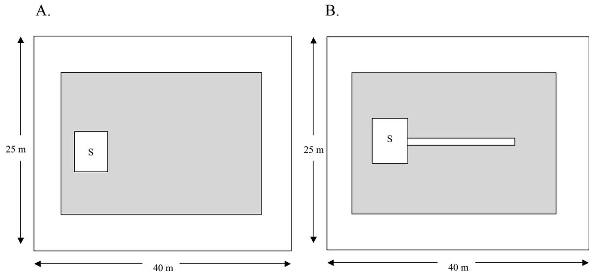
**Figure 17.** Schematic design of; A.) a typical 1,000 m<sup>2</sup> marron grow-out pond with 3 x 3 m concrete sump (S); B.) a 1,000 m<sup>2</sup> large nursery pond constructed at the Pemberton Freshwater Research Centre to support the current project, with a 3 x 3 m concrete sump (S) and a 9.6 m concrete channel to allow the aggregation of large numbers of juvenile marron. From Molony (2002c).
