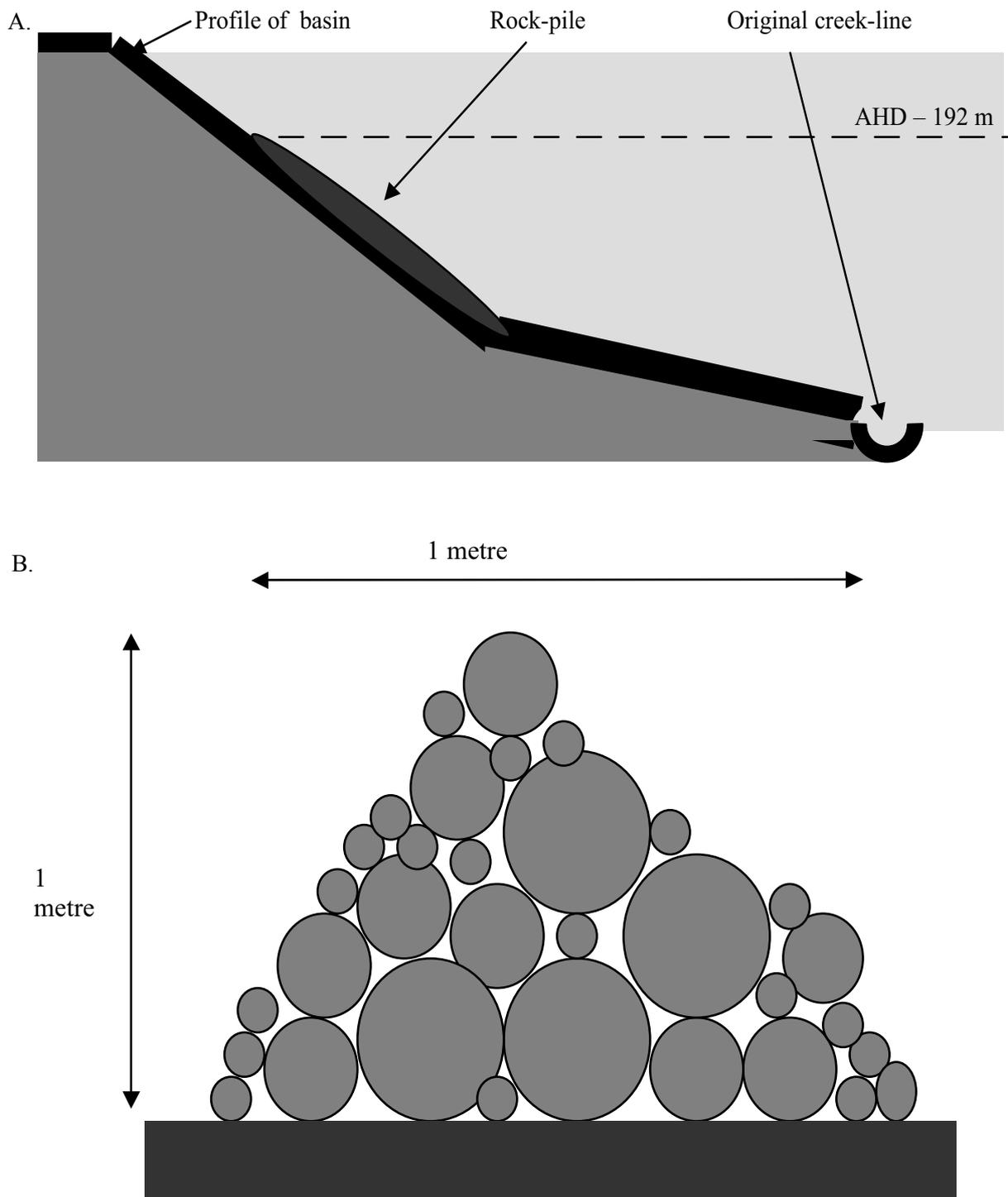
**Figure 28.** Generalised design of the rock-line artificial habitats installed at Lake Navarino. A). Profile of position of a rock-pile. Linear distances varied among rock-piles, 20-100 m long; B). Stylised cross-section of a rock-pile demonstrating the large number and random position of holes and crevices of the structures.
