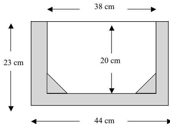
**Figure 18.** Details of the cross-section of the 9.6 m concrete drain available as 'small spoon drain section' from many concrete product manufacturers in 1.2 m lengths. From Molony (2002c).
