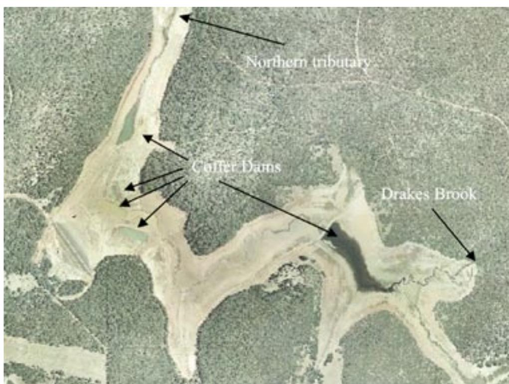
**Figure 2.** Aerial shot of the drained basin of Lake Navarino in Autumn 2003, showing location of the substantial coffer dams present and the two perennial tributaries.
