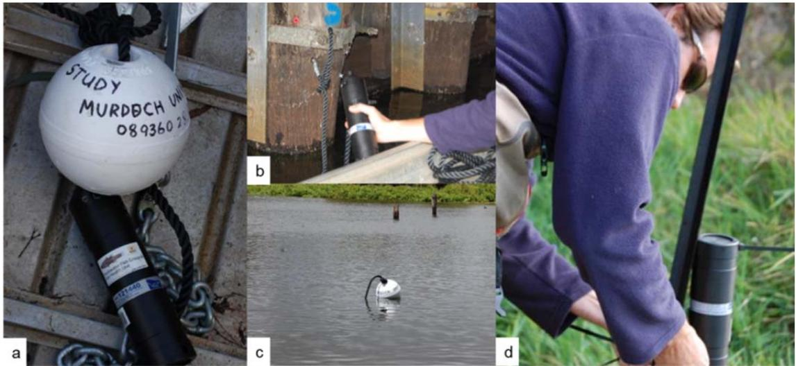
**Fig. 6:** (a) VR2W acoustic receiver unit attached to styrene float/sand anchor mooring prior to deployment; (b) deployment of receiver attached by rope to bridge infrastructure; (c) styrene float/sand anchor mooring deployment; (d) deployment of receiver attached by cable ties to metal stake (New River Wetland).
